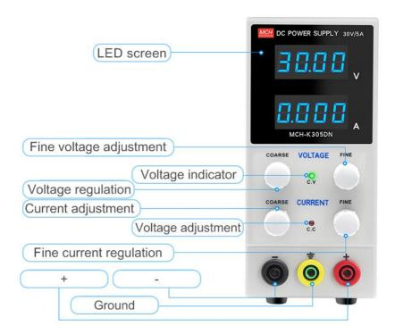
Note: When the current through the load (calculated according to Ohm's law) is lower than the preset current value, C.V lights, then the power supply works in constant voltage mode. Otherwise C.C light, then the power supply in constant current mode, through the load current is limited to the preset current value. That is, the load current is greater than the power supply current, work in constant current mode.
